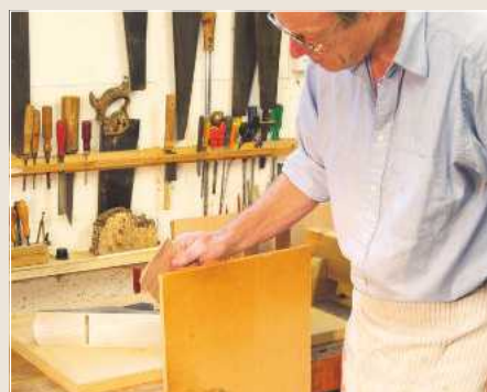
▲ Pic.5 The corners will need to be smoothed with abrasive paper from the outside towards the centre
